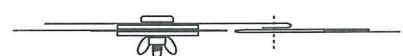
5" FLAP ONE ROW OF LOCKSTITCH AT 4 STITCHES PER INCH. MATERIAL PVC MESH.
